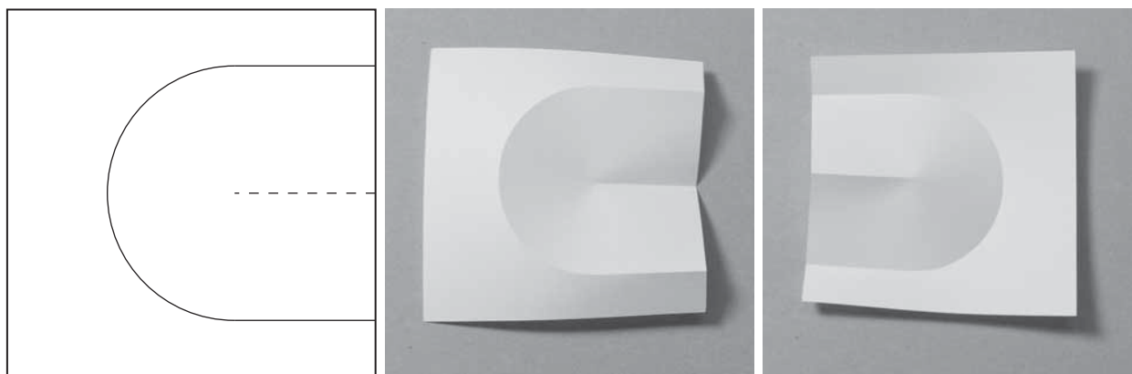
Figure 5.9 Crease pattern to fold a part of the cone and the resulting shape (right: backside).
