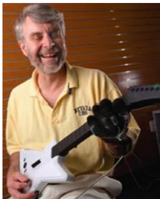
Fig. 8 Haptic feedback glove adapted to play Guitar Hero for the visually impaired
